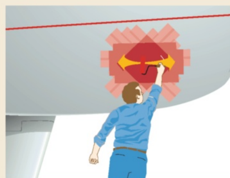
C) ...finishing with horizontal strokes to align any brush or roller marks with the water flow
